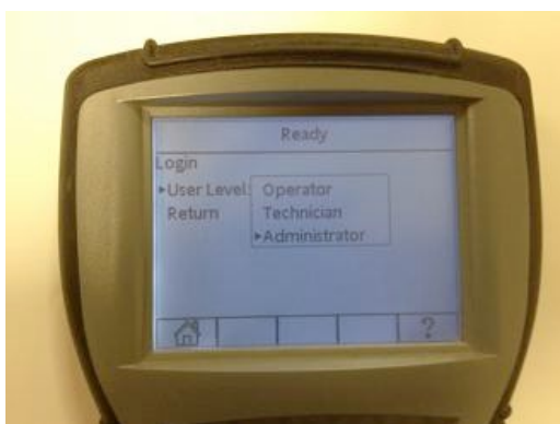
7. Select Administrator and Press Enter. If a password is required, password will be 2222 or any password you have assigned. Press F1 for the Home Screen.
